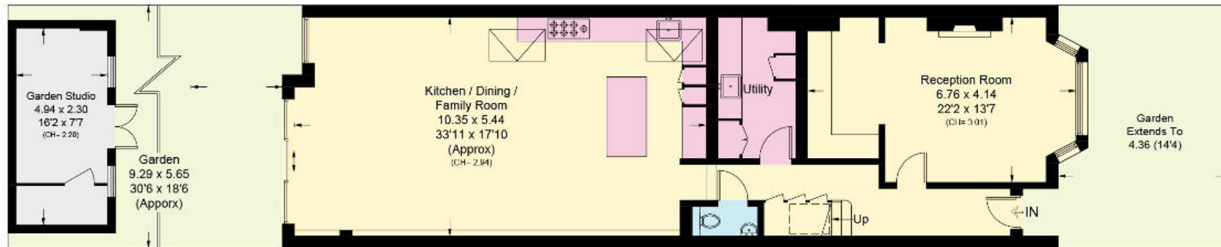
Ground Floor Approximate Area = 104.5 sq m / 1125 sq ft Including Limited Use Area (0.9 sq m / 10 sq ft)
